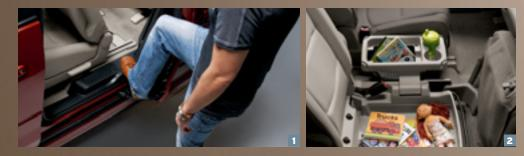
1 One-Touch "Walk-In" Feature. With one touch, second-row seats slide and seatbacks tilt forward to allow easier third-row access. The MAZDA 5's two large, perfectly balanced rear doors slide open with ease—a real convenience in a tight parking space. 2 A Second-Row Foldout Table with built-in dual cup holders, storage bin and under-cushion storage is center-mounted for maximum utility and passenger convenience.
