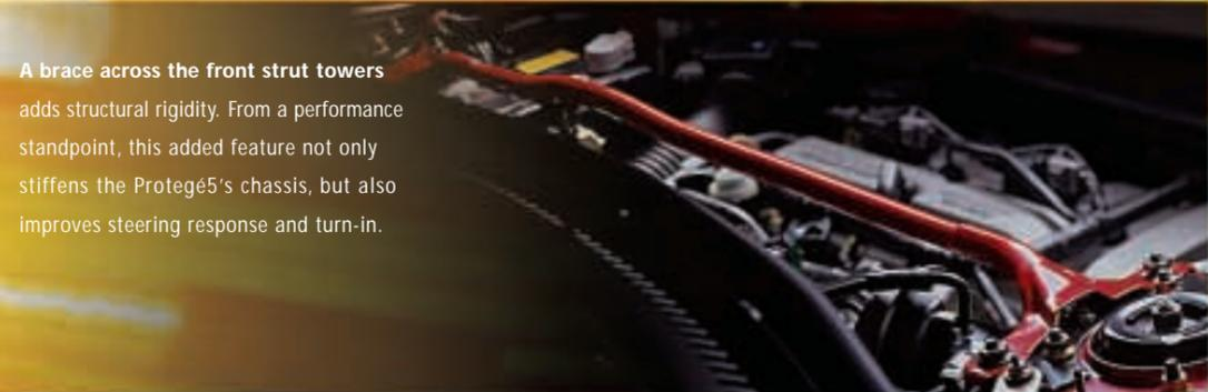
A brace across the front strut towers adds structural rigidity. From a performance standpoint, this added feature not only stiffens the Protegé5's chassis, but also improves steering response and turn-in.
