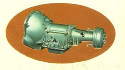
The Chrysler PowerFlite fully automatic transmission combines with the Spitfire V-8 engine to give you superlative break-away and acceleration throughout the entire power range. Power-Flite gives the highest torque multiplication. It is simpler in design. Has fewer parts. It is lighter in weight. And it is fully automatic. With the new, exclusive Push-Button Selector, you merely push the button for the driving range you want — no gearshift lever!
