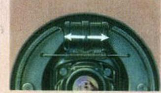
Chrysler's centrifuse brake drums present a cast iron braking surface which resists scoring and prolongs the life of linings. Fins on the steel casing aid in cooling.
