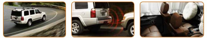
Commander's standard ParkSense® Rear Park Assist System<sup>®</sup> helps to make sure you back into and out of your parking space safely. Ultrasonic sound waves give an audible and visual warning when driving in reverse at speeds below 10 mph. Advanced driver and front-passenger multistage air bags<sup>®</sup> and Side Occupant Protection System with side-curtain air bags<sup>®</sup> help protect Commander's outboard occupants.
