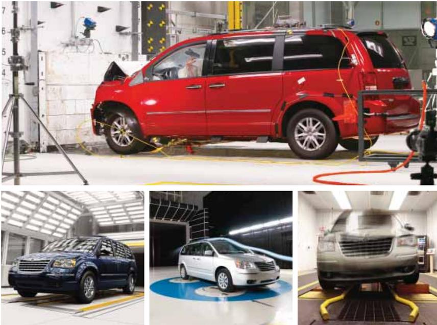
Top: Town & Country testing in action during a high-speed crash test. From left, functionality evaluations under extreme temperatures, improving aerodynamics with the help of a 100-mph wind tunnel, and working out NVH kinks on the four-post shaker.
