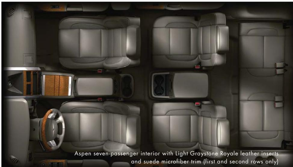
SEVEN-PASSENGER bucket seating. Two bucket seats in the second row and three-passenger 60/40 split-folding bench seating in the third row.
