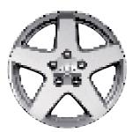
NEW 20" Chrome- clad Cast Aluminum Wheel Optional on SLT "G" and Limited Models
