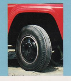
Tight turns. Widetrack front axles with large wheel-cut angles allow sharp-turning maneuverability.
