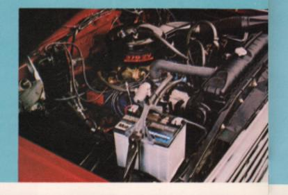
Service ease. Ford's long conventional hood opens high and wide for easy access. And the engine is entirely ahead of the cowl so service points, spark plugs and accessories are easy to reach.
