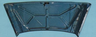
Built tough. All Ford F-Series trucks have sturdy reinforced steel cabs. The broad alligator hood has double-panel sections to minimize flutter. Doors have double-panel construction, too.
