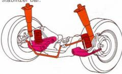
The rear suspension features a four-bar link system with coil springs. Coupled with the hybrid strut front suspension, Fairmont handles tight turns with hardly any body lean. The weight is maintained on all four tires throughout the turn. Especially helpful in congested city traffic where quick, tight turns are often required.
