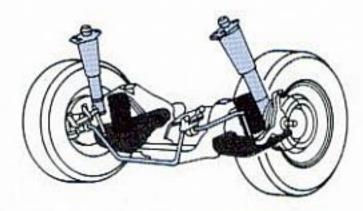
The Fairmont front suspension is a hybrid strut-type suspension, using one ball joint, one control arm, a coil spring and a strut. A system specially engineered for Fairmont. With computer-selected coil springs and vertically-mounted shock absorbers to help provide control on rough city streets.
