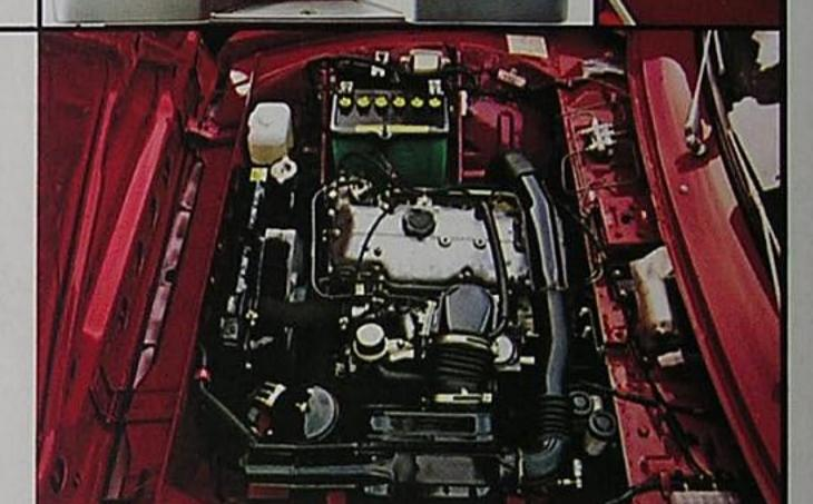
Big 4-cylinder, 1800-cc. displacement engine provides plenty of pep and power, Construction features include full-circle water Jackets, cast iron cylinder block, cast aluminum cylinder head and valve cover, full pressure lubrication and large capacity oil pan. Standard four-on-the-floor transmission is synchronized in all forward speeds. Short-throw design gives fast, easy shifting.
