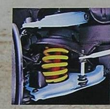
Independent front suspension. Each front wheel rolls over bumps independently. Jolts and jars are absorbed by big coil springs and shock absorbers. Front stabilizer bar reduces roll and sway. Long 104.3-inch wheelbase spaces out and dampens down bumps for a smooth ride.
