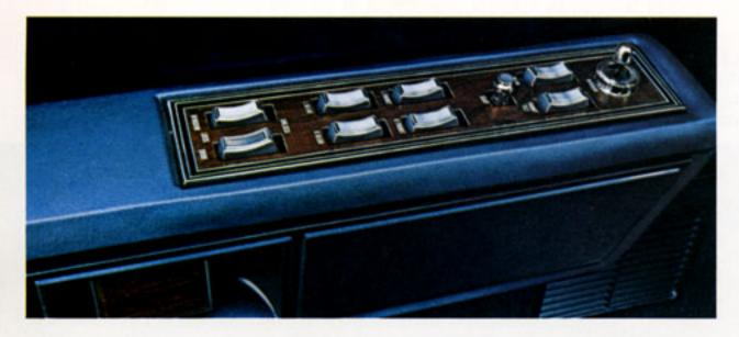
Power control panel in driver's padded armrest has easy-to-reach switches (left to right) for window and door locks; power windows; power seat control; and remote control outside mirror. Below the armrest, a door-mounted speaker, a feature included with all Lincoln Continental optional sound systems.
