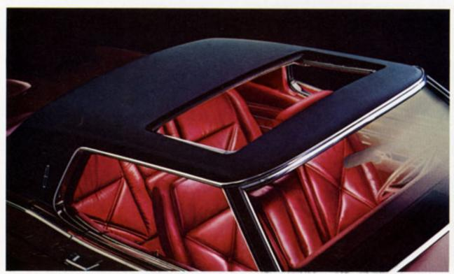
Power-operated sun roof (shown on Mark III) gives you the exhilarating feeling of an open car without the drafts all around you. From an instrument panel switch, which acts as a positive roof lock, you can control the roof panel's rearward movement for any opening up to 21 inches deep by 36 inches wide.
