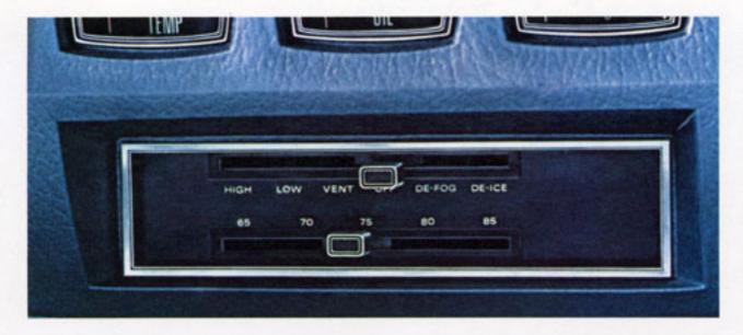
Automatic Temperature Control is standard on every Lincoln Continental. This sophisticated year-round air conditioning/heating system cools or warms rapidly to within a degree or two of the temperature you pre-select. And maintains this environment without any further manual adjustment. The air conditioner dehumidifies as it cools. Can remove pollen and dust from incoming air. At the touch of a switch, it can defog or de-ice the windshield.
