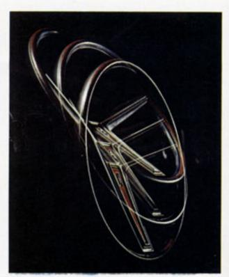
Tilt steering wheel. Adjusts to five positions through a 30-degree arc, so any driver can select his most restful driving angle. The tilt wheel also permits easier entrance and exit.
