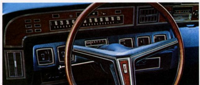
The beautifully organized instrument cluster places most-read dials in the driver's line of sight, and most-used buttons within easy reach. Just left of the drum-type speedometer is a signal light bank that can give you instant reports if the headlamp doors are closed, fuel is low or dual brake system has a loss in hydraulic pressure. Also, seat belt warning light.
