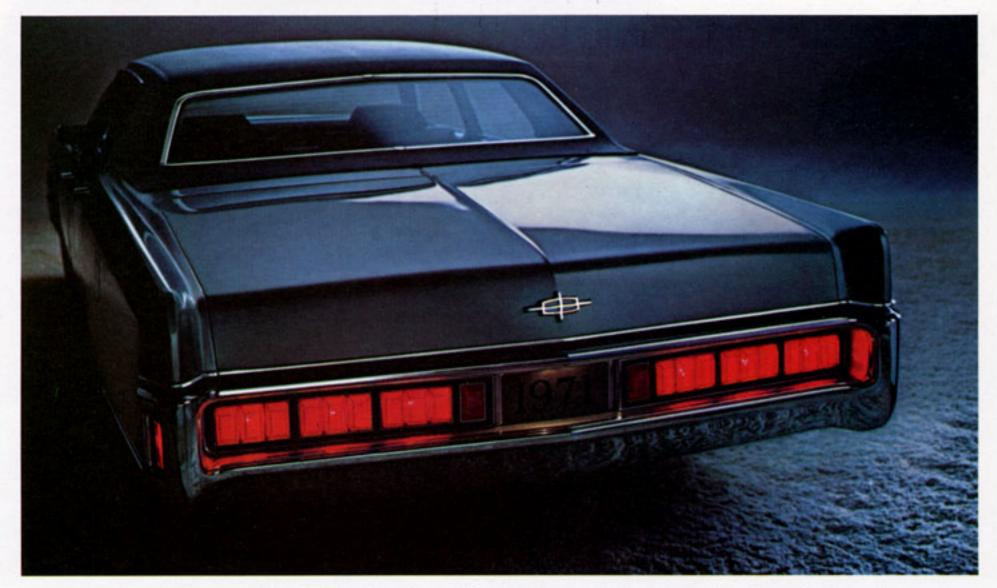
New taillight assembly reflects Lincoln Continental's traditional understated elegance. Backup lights flank the license plate. The fine, almost invisible lines in the rear window are heating elements for your optional rear window defroster.
