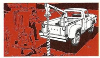
REAR-MOUNTED PTO-DRIVEN mobile worksavers, such as post-hole diggers, feed mills, saw mills, hay balers, and many other gear, belt or hydraulically actuated attachments may be easily installed.
