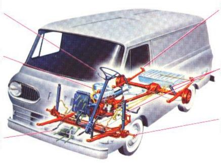
Durable, soft-action rear suspension with variable-rate, semielliptic leaf springs.
