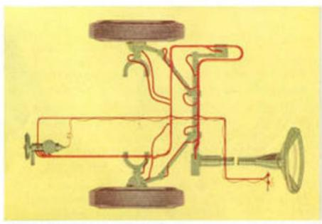
Lincoln Push-Button Lubrication gives you proper lubrication of front-end suspension and steering at just the push of a button. This power-operated system has a reservoir which holds grease for from 250 to 300 lubrications. No matter how dusty the weather, your Lincoln will be properly lubricated, keep that "new car feel" longer. A Lincoln "first," optional at moderate extra cost.
