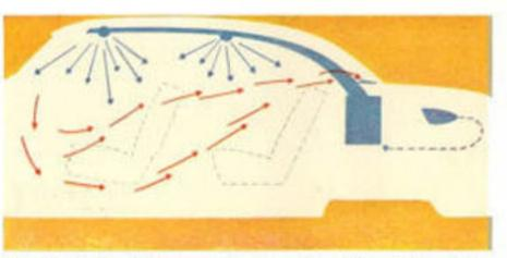
Lincoln Air Conditioning cools, cleans, dehumidifies and circulates up to 258 cubic feet of air per minute—gives you perfect comfort no matter how hot the weather. There are four air inlets, one over each door, controlled by individual louvers.
