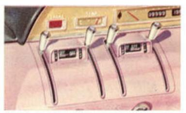
Lincoln Dual-Control Heater combines an underseat beater with a front compartment heater, which can be operated separately to get the desired degree of warmth. A two-speed blower circulates air, defrosts windshield,
