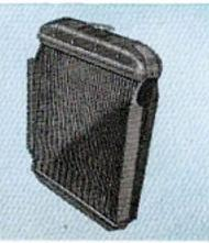
Sturdy, heavy-duty radiator with a highspeed fan improves engine cooling under all idling or operating conditions. Standard with Interceptor, available at extra cost with V-8 or Six.
