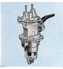
Combination fuel and vacuum pump offers positive windshield Wiper operation. (Standard with the Interceptor V-8 and with Fordomatic or Overdrive.)
