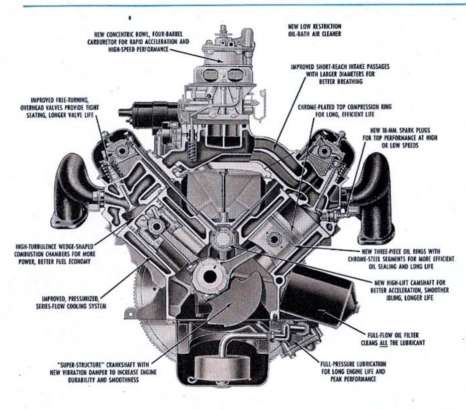
NEW INTERCEPTOR V-8 WITH HIGH-COMPRESSION, SHORT-STROKE, LOW-FRICTION DESIGN FOR TRIGGER-TORQUE PERFORMANCE
