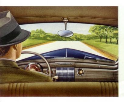
To see the world and more of it! The Lincoln-Zephyr Panorama windshield is one broad, deep piece of glass—you see greater stretches of road and landscape. Ventilating wings are built into front side windows; they are opened and closed by regulator handles. Push-button locks are on each door.
