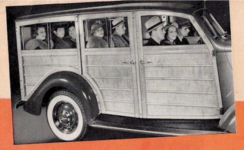
Front and rear seats each accommodate three. The center seat is double width, leaving ready access to rear. Rear seat can replace center seat, providing room for six with unusually large luggage space, or both center and rear seats can be removed completely.
