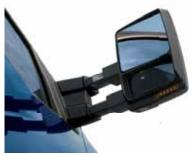
**TRAILER TOW MIRRORS** manually telescope and fold forward or backward so you can get through tight spaces. Whether you're towing or not, the large viewing area and convex lens on these available mirrors help improve visibility and reduce blind spots.
