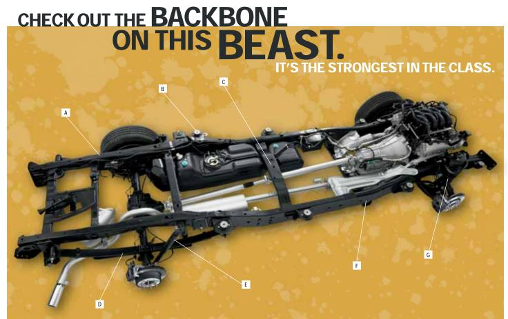
STRONGEST FRAME IN THE CLASS (A) is the backbone of F-150's class-leading capabilities. The fully boxed, ladder-style frame also contributes to the quiet interior and controlled ride.
