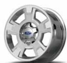
17" 7-Lug Steel Included with Heavy-Duty Payload Package
