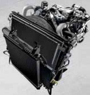
**COMPREHENSIVE COOLING:** The engine radiator in this cooling system is especially large, and the high-flow water pump efficiently moves coolant. There are 6 different radiators — including one for the fuel cooling system — designed to support engine emissions and enhance durability, power and torque benefits. An engine-mounted fan shroud improves airflow efficiency, resulting in an overall cooling system that is capable and reliable, especially under extreme towing demands.
