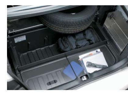
CAUTION: Do not place stiff or sharp objects in the trunk that could be pushed forward into the fuel tank in a high-speed rear impact.
