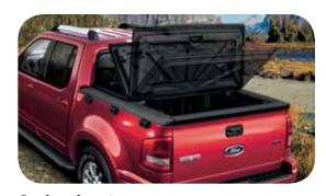
**3 simple steps** The optional, locking hard tonneau cover is hinged in the middle, so you can access just the front or back of the box, as needed. Want to access the entire thing? The tonneau cover can be removed in just 3 steps.
