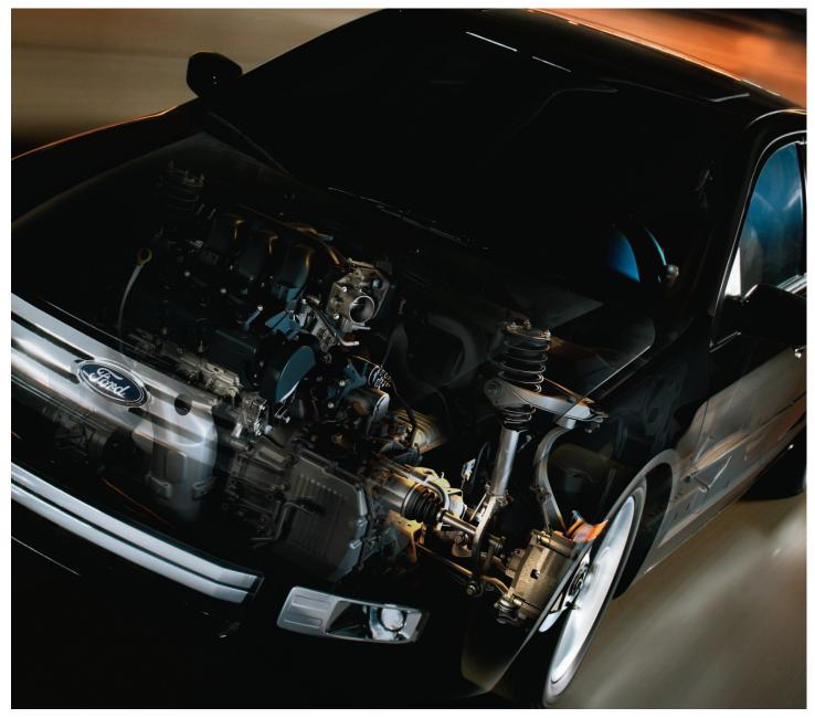
The 4-wheel independent suspension keeps chassis motion and body roll to a minimum with help from front and rear stabilizer bars. And control through the turns means – you guessed it – responsive driving. Gotta love that.
