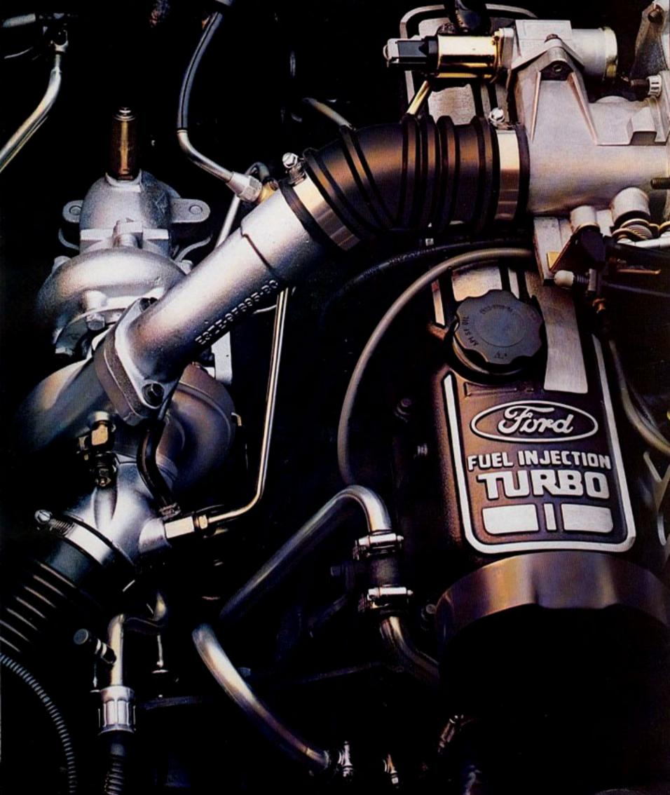
ougar's sophisticated technology expresses itself under the hood in each of three available engines. All are equipped with standard electronic fuel injection (EFI) and fourth-generation Electronic Engine Controls (EEC-IV).
