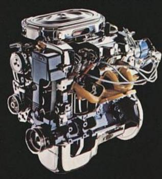
(3) Central spark plug location creating a direct power charge for efficient combustion.
